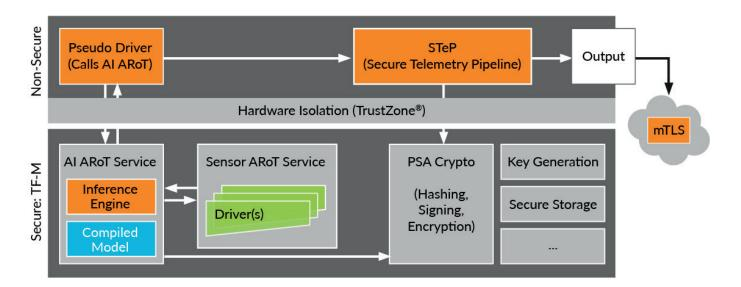
If secure data storage is required to be stored off-chip, data can be encrypted using a device-bound encryption key derived from a hardware unique key (HUK).
